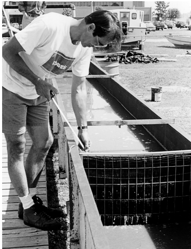
Figure 2.1 Testing Silt Fence Performance in a Flume
