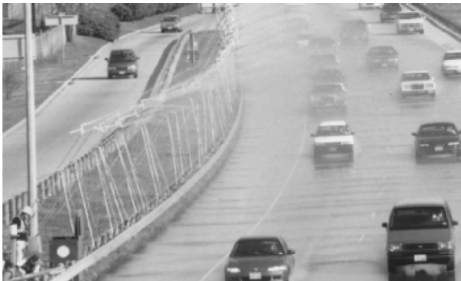
Figure 5.1 Rainfall Simulator in Operation
