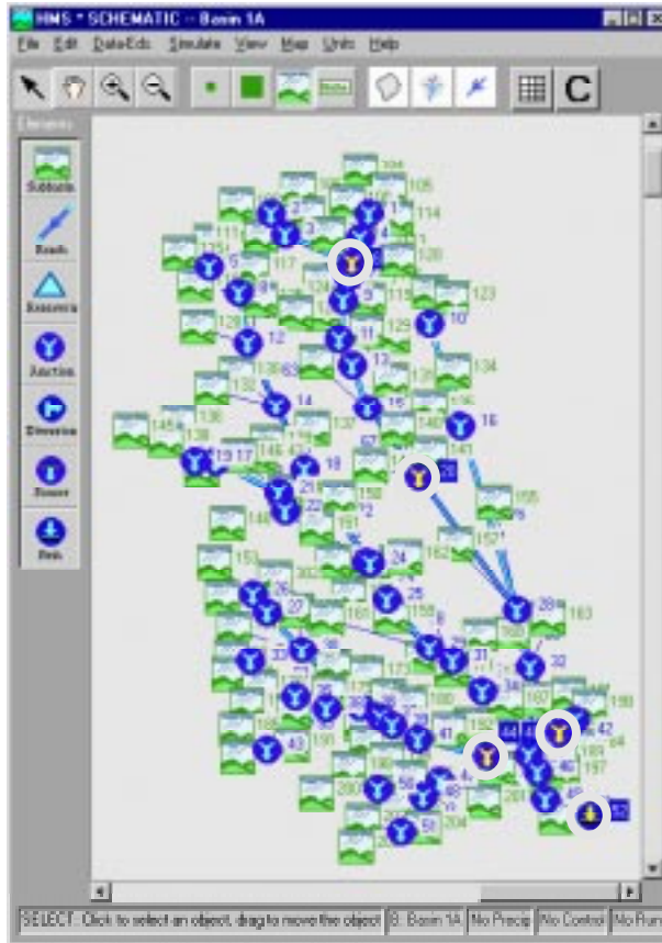
Figure 23: Basin Schematic Showing Linked Junctions (highlighted in yellow)
